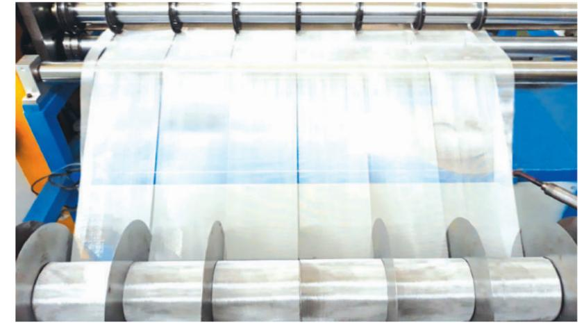
It is shearing operation that cut a large roll of meshes into narrower rolls. We can decide the size depending on customer's requirements.
