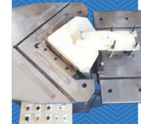
Pressing is the process of placing flat sheet metal in either blank or coil form into a stamping press where a tool and die surface forms the metal into a net shape. The pressed products can be used for filters and parts of vehicle.
