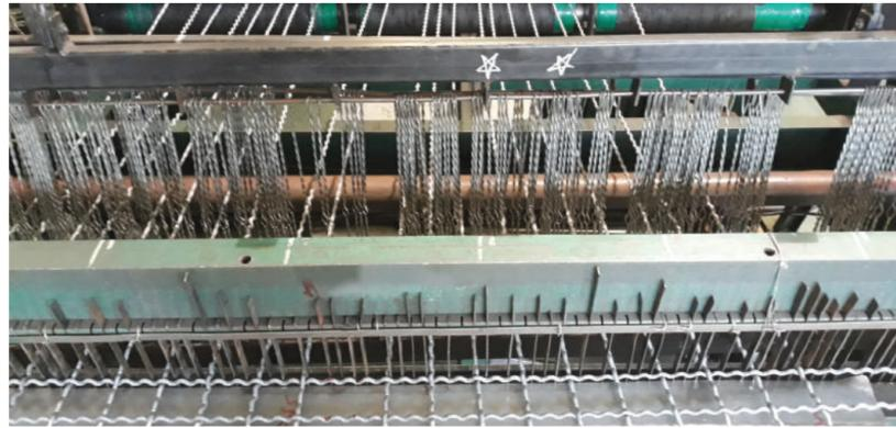
Crimped Wire Mesh is constructed of wires that have been crimped prior to weaving them together in a loom. Crimping the wires before weaving provides stability and consistency in larger spaced wire mesh. It also can be produced with numerous sizes.
